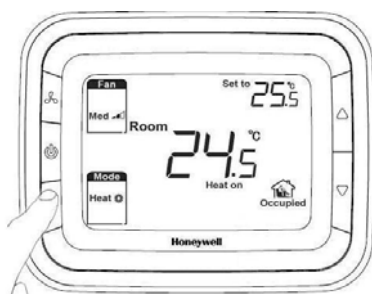
PRESS THE MODE BUTTON TO SELECT HEAT, COOL, OR VENT
